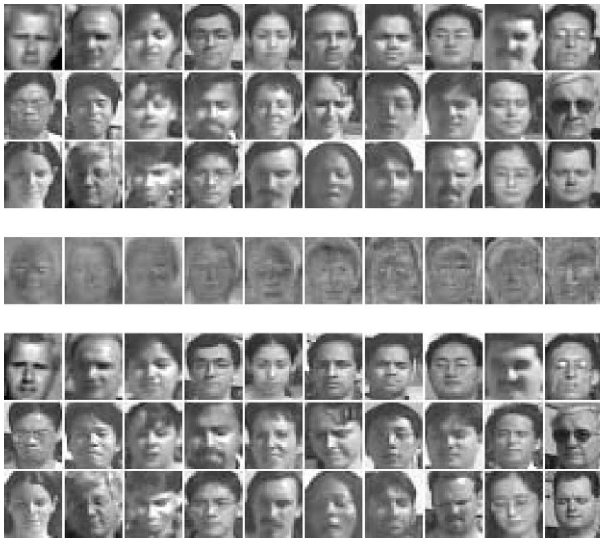
Fig. 7. Database-1. Top row: the second facial images for training probabilistic density. Middle row: top 10 eigenvectors for the IPS. Bottom row: the facial images cropped out from the largest frontal view.
