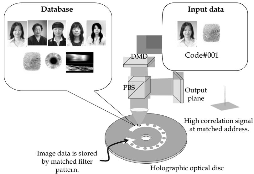
Figure 25. Concept of optical correlator based on optical disc
