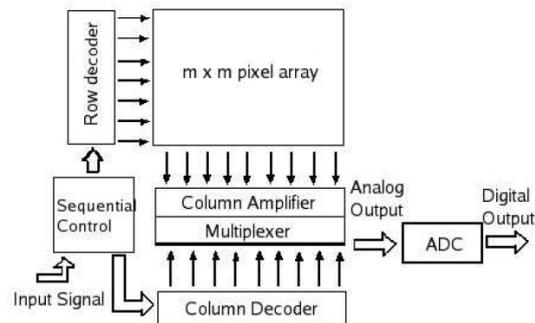
Figure 9. Image Sensor Architecture
