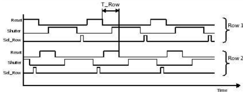
Figure 12. Timing diagram of the rows control signals
