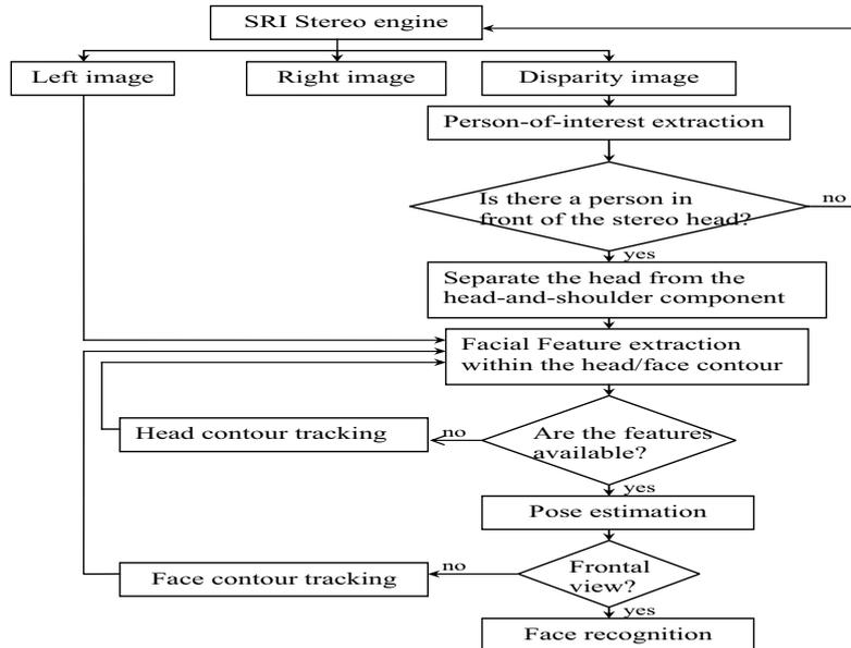
Figure 1. Flowchart of the head/face tracking algorithm
