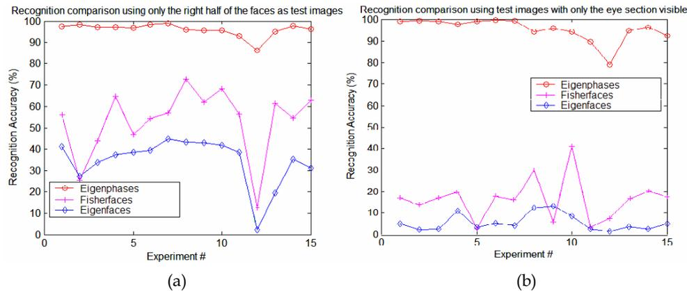
Figure 5. Rank-1 identification rates obtained by *Eigenphases*, *Eigenfaces*, and *Fisherfaces* for two different experiments each using different types of partial faces. (a) right half face (b) eye-section face
