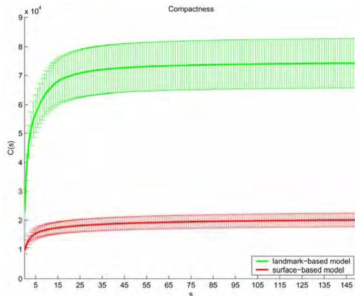
Figure 11. The compactness scores of the landmark-based and surface-based models. The standard error bars indicate the likely error of  $C(s)$  allowing one once more to conclude that there is significant difference between the compactness scores of the two models
