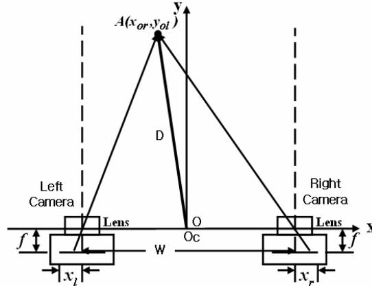
Figure 2. Structure of a parallel stereo camera
