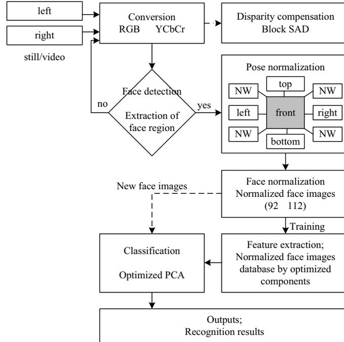
Figure 1. Block diagram of the proposed algorithm
