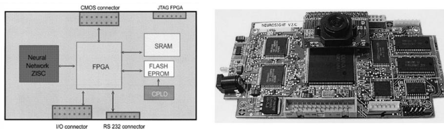
Figure 6. Neurosight block diagram and board picture
