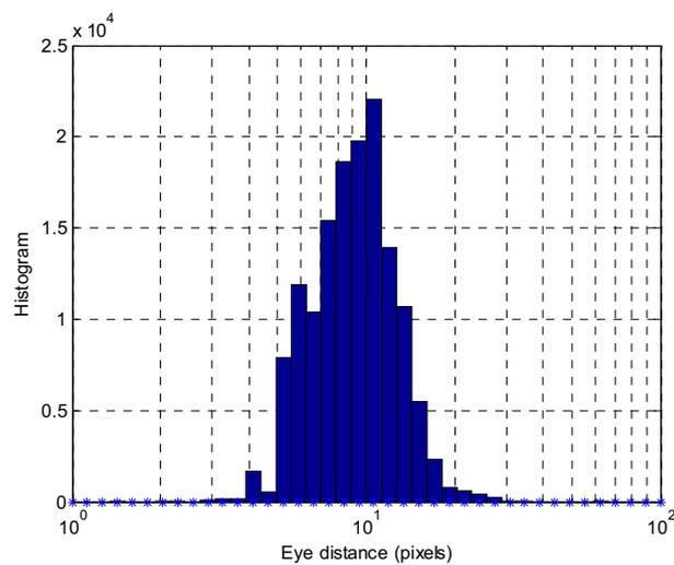
Figure 2. Histogram of the eye distances of the faces segmented from the probe videos using the manual annotations. The video-to-video face recognition system has to cope with eye distances of 4 to 28 pixels
