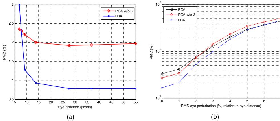
Figure 4. Effect of far-field viewing conditions on linear subspace projection face recognition. (a) Performance as a function of face resolution. (b) Performance as a function of eye misalignment
