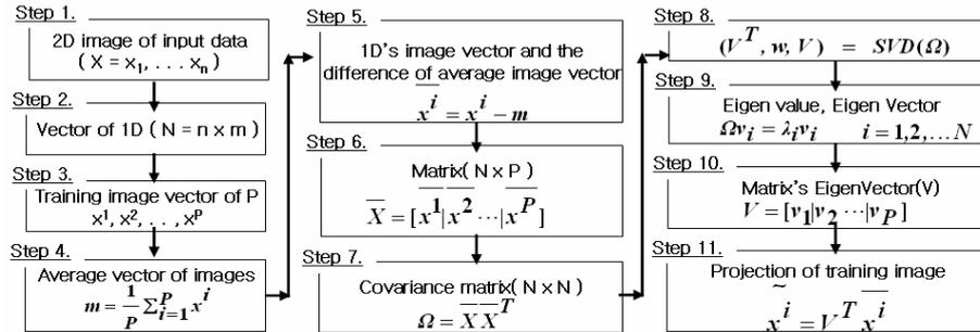
Figure 8. The block diagram of PCA algorithm
