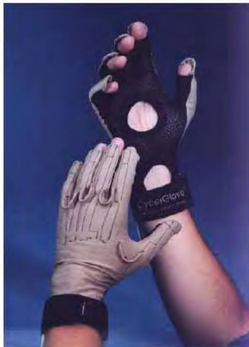
Figure 5. The 'CyberGlove' for hand gesture recognition [Blinghurst, 2002]
