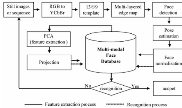
Figure 1. Face feature extraction and recognition process
