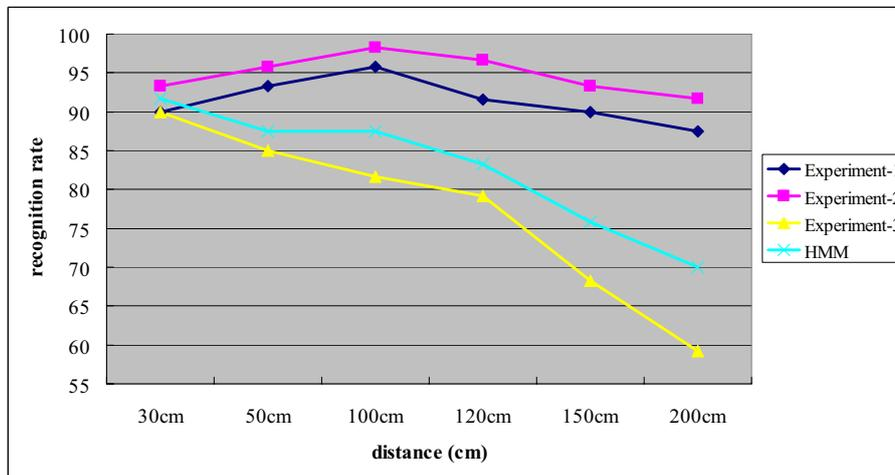
Figure 14. Recognition rates versus distance comparison for the proposed and various existing methods
