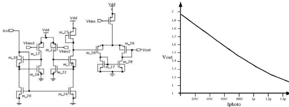
Figure 11. Column amplifier schematic and simulation results
