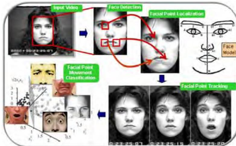
Figure 7. Outline of the AU recognition system of Valstar and Pantic (2006a)
