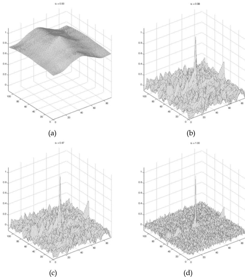
Figure 10. Mesh plots of correlation planes produced from application of OTSDF filter expecting AWGN of SNR 20 dB to a training image with varying values of  $\alpha$  (a)  $\alpha = 0$  (b)  $\alpha = 0.33$  (c)  $\alpha = 0.67$  (d)  $\alpha = 1.00$
