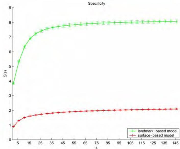
Figure 10. The specificity scores of the landmark-based and surface-based models. Small standard error in  $S(s)$  (as shown from the error bars) also allows for us to conclude safely that the difference in specificity scores is indeed significant
