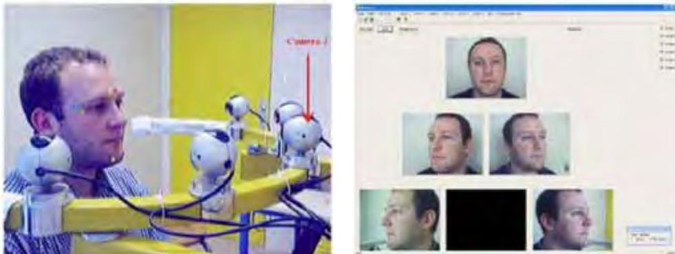
Figure 16. Acquisition system with 5 cameras and example of 5 images collected from a subject
