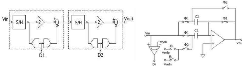
Figure 13. Pipeline ADC Architecture and Associated Circuit
