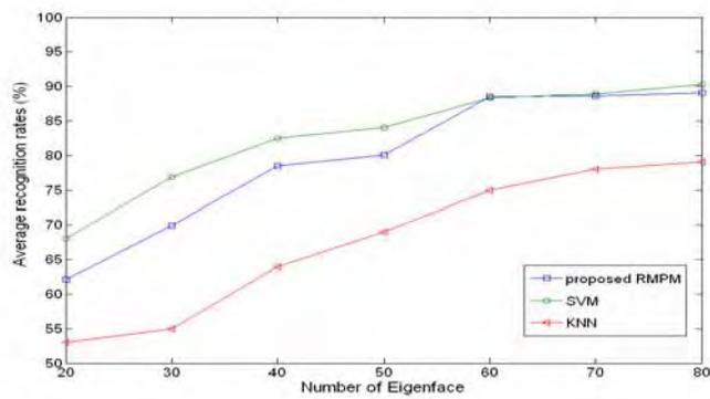
Figure 11. Recognition rates for **2D** vs. number of eigenfaces on XM2VTS database
