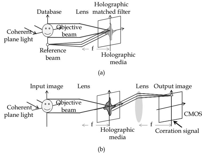
Figure 1. Concept for a matched filtering correlation in FARCO system: (a) Recording a matched filter, (b) Filtering (Optical correlation) process
