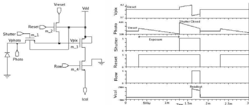
Figure 10. Pixel circuit schematic and results of simulation
