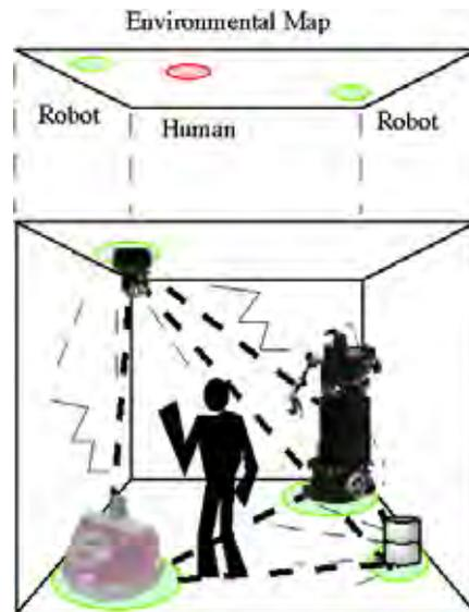
Figure 3. The sensor network among robots and their environmental system
