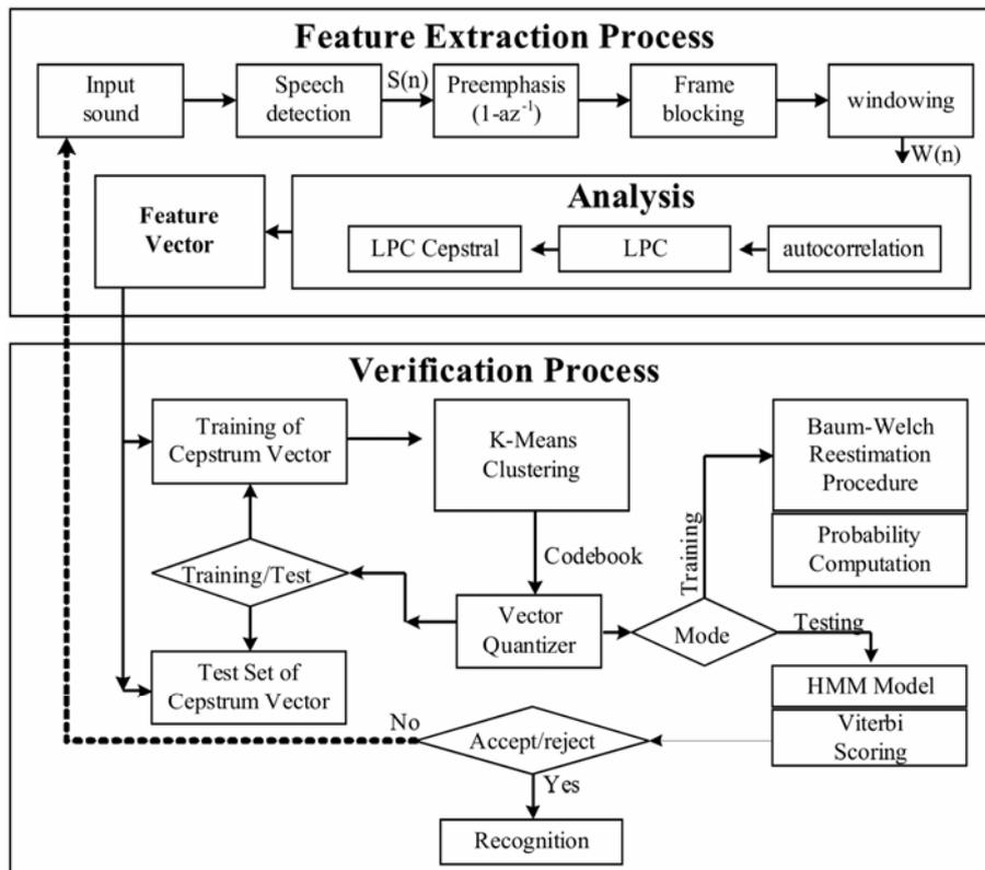
Figure 6. Feature extraction and verification for speech
