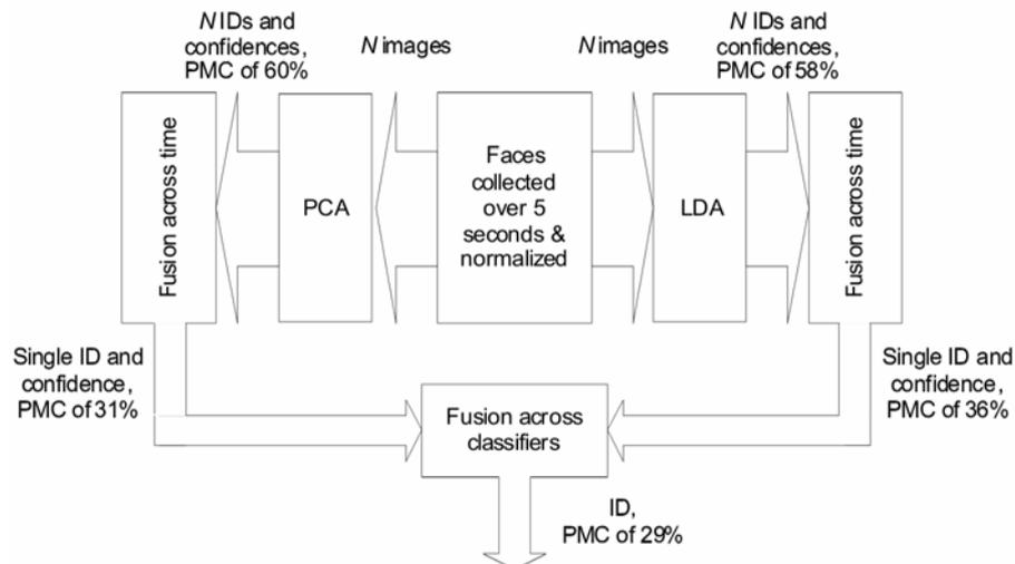
Figure 7. Two-stage fusion scheme. The PMC shown at the various stages of the scheme correspond to the 15 sec gallery videos, face extraction using the provided annotations and classifying the extracted probe stills according to the distance from the gallery class centres. The individual decisions for the probe faces are fused using the sum rule (Kittler et al., 1998). According to the sum rule, each of the decision  $ID_i$  of the probe faces in a testing
