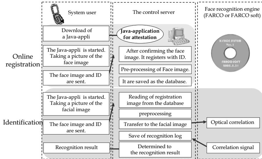
Figure 18. Block diagram of cellular phone face recognition system
